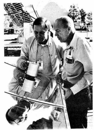
TAKING THE MEASURE of a solar collector mirror are, from left, Jim Freese (2525) and Lew Larsen (4716). They're using the new portable specular reflectometer developed by a Dallas firm under a Sandia contract. The device measures how the reflectance of a mirror surface is affected by
